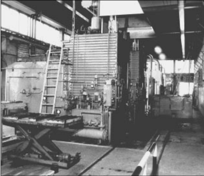
Figure 4. Example of furnace and charging (above). The parts are loaded in baskets or on fixtures (at right) before they are taken to and loaded into the furnace by means of a car.
