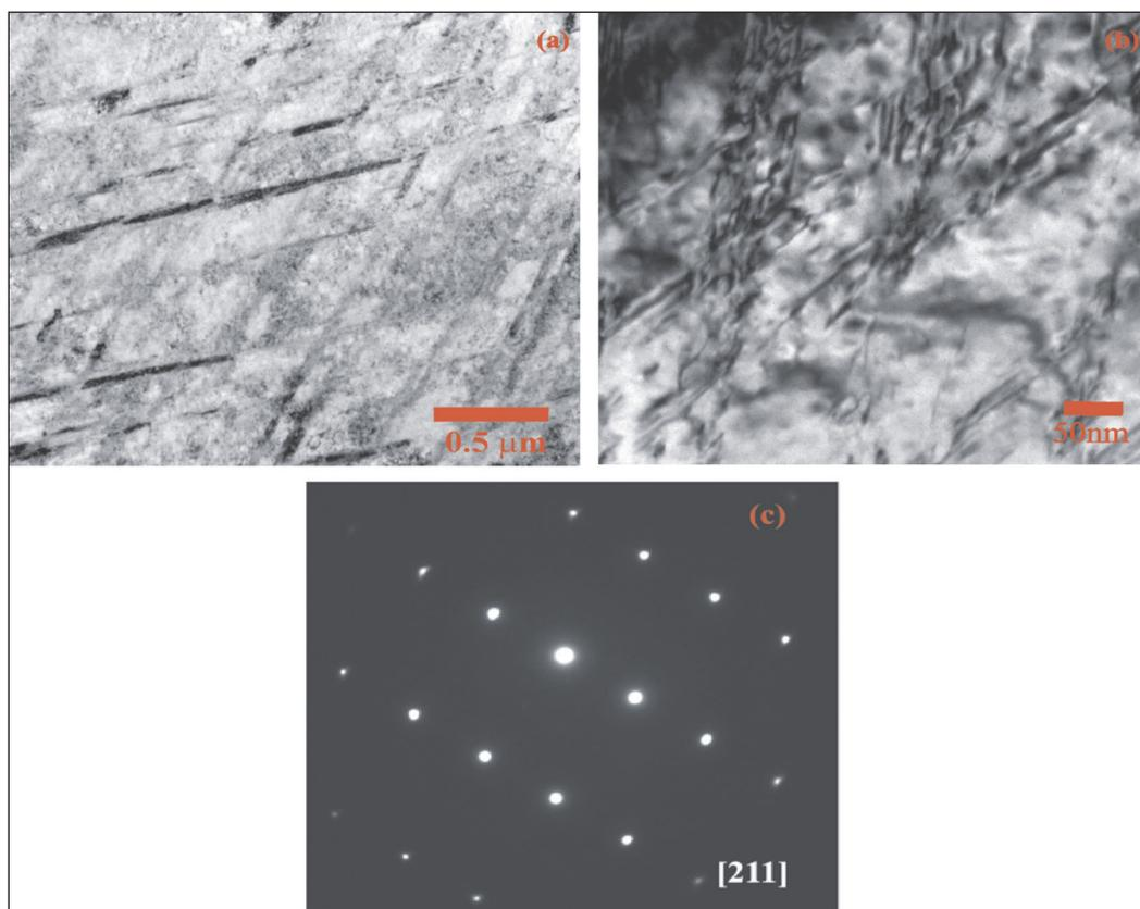
**Fig. 6 : Bright field micrographs of samples deformed at 923K in 1073K/8h aged condition at a strain rate of  $8.3 \cdot 10^{-3} \text{s}^{-1}$  (a) multiple slip with high dislocation density in the matrix (b) heavy deformation of matrix in between the slip bands indicating the presence of dislocation tangles, dislocation loops, dislocation pairs and dislocation dipoles (c) bright field image shown in (b) was obtained using [110] zone axis.[9].**
