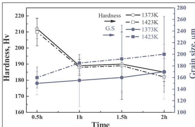
**Fig. 1 : Variation in grain size and hardness of solutionised samples of Superni 263 alloy as a combined function of time and temperature**
