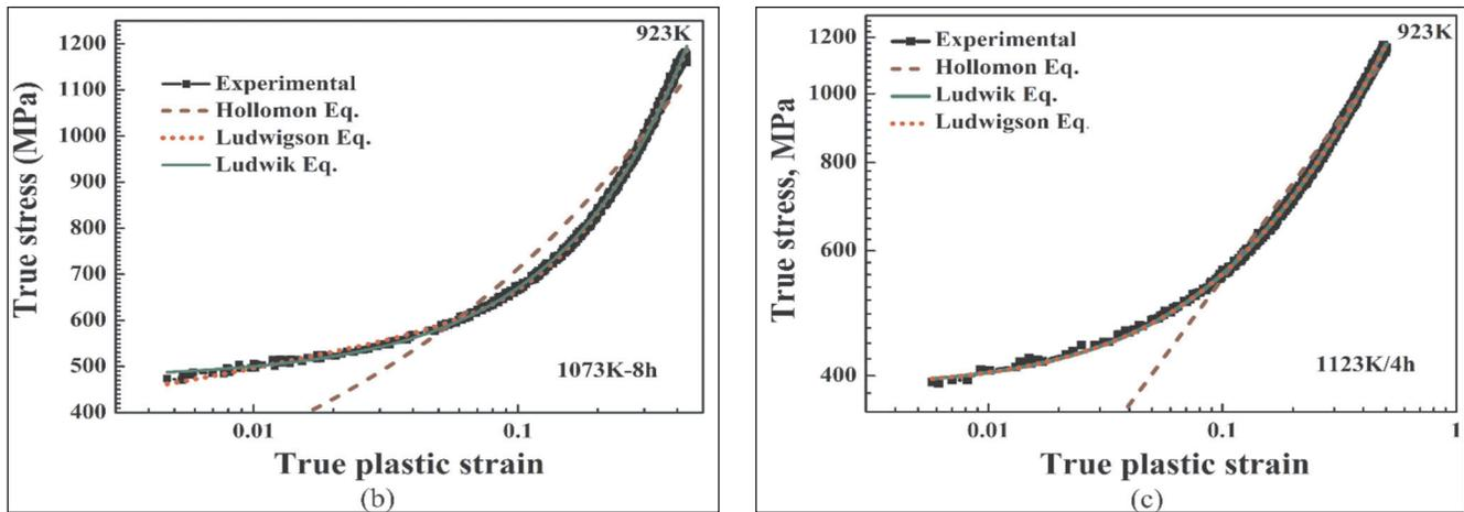
**Fig. 4 : True stress-true plastic strain data of Superni 263 alloy fitted with various flow relationships in three aged conditions at 923K.**
