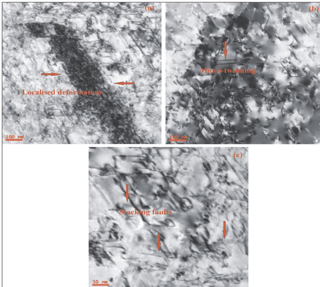
**Fig. 7 : TEM bright field micrographs of deformed samples at 923K (1123K/4h) aged (a) localization of deformation in planar slip band (b) micro twinning and (c) stacking faults [9]**
