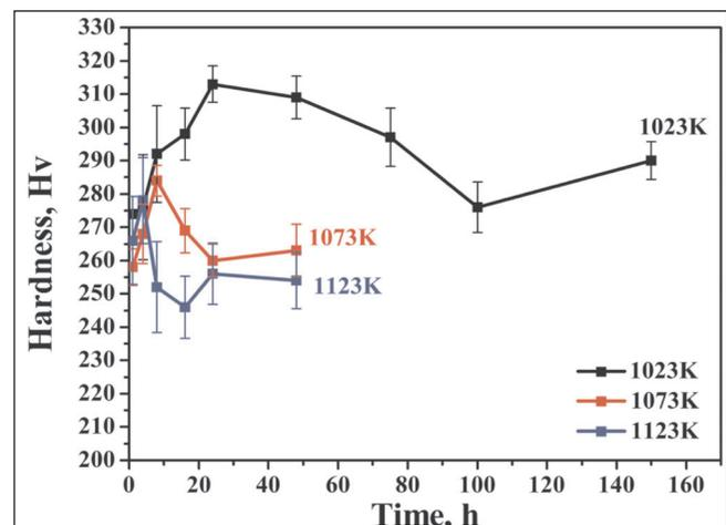
**Fig. 2 : Variation of hardness of Superni 263 alloy as a function of aging duration at 1023K, 1073K and 1123K.**
