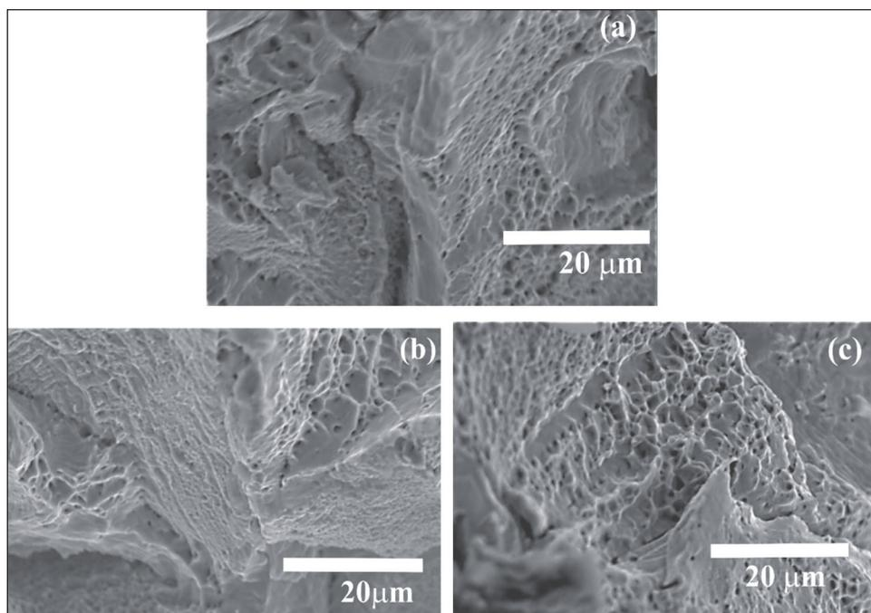
**Fig. 5 : Tensile fractographs of Superni 263 alloy tested at 923K, in all peak aged conditions, illustrating (a) long intergranular cracks with mixed mode fracture at (1023K/24h) (b&c) Shows ductile fracture with isolated cavities from the discrete carbides and no linking of the cavities.**
