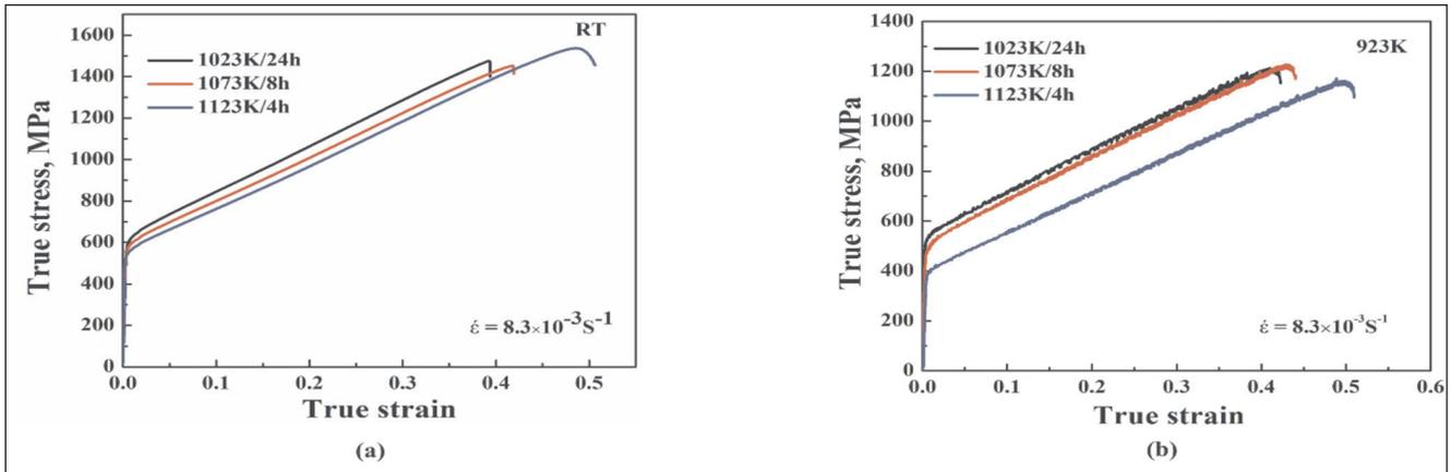
**Fig. 3 : True stress-true strain plots of SU-263 alloy in different aging conditions that gave peak strength on aging at 1023K,1073K and 1123K ( $\dot{\epsilon} = 8.3 \times 10^{-3} \text{ s}^{-1}$  at 298K and 923K ).**
