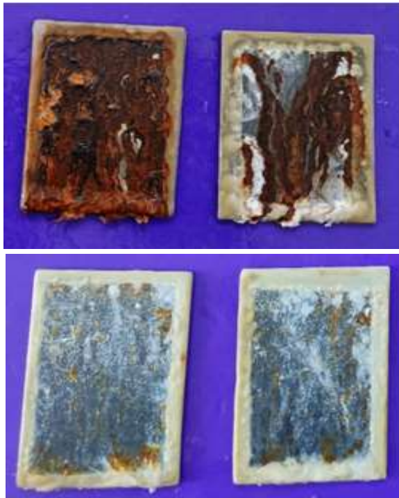
Figure 11 Comparison salt fog exposed coated panel (a) plain zinc coating and (b) Zn-0.02Sr Coating.
