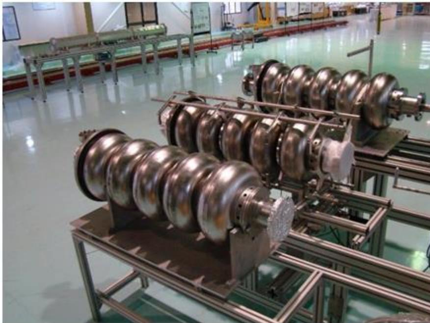
**Fig.2** Vacuum cavities prepared in DAE and provide US national labs for accelerators.
